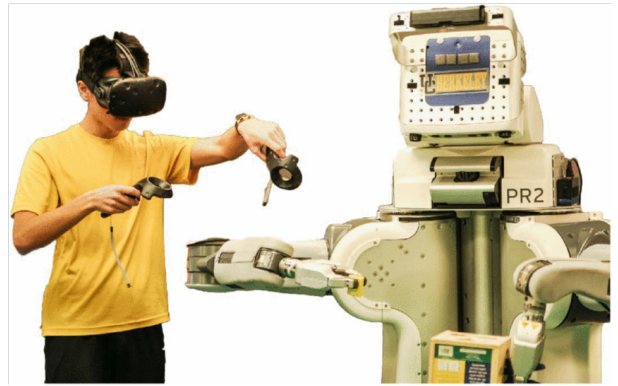
Fig. 1. Virtual Reality Teleoperation for Imitation Learning (i) with PR2 Robot mounted with RGB-D camera, (ii) human operator operating using VR headset and two VR hand controllers [1].
